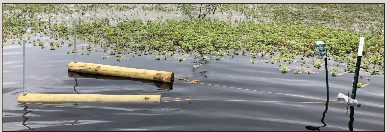
FIG. 3. Photograph (viewed from the side) of a camera-trap basking array designed to detect the presence of Western Chicken Turtles ( Deirochelys reticularia miaria ).
