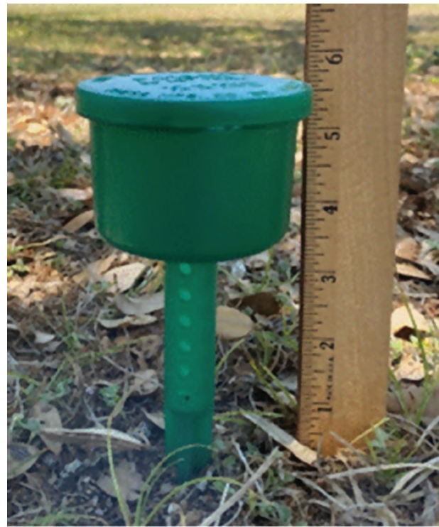
Fig. 1. Ants-No-More Bait Station includes a covered cup to hold bait and a porous stalk where the bait is available to foraging RIFA.
