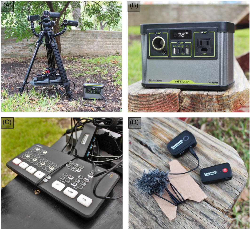
FIGURE 2 Cameras and tripod connected to battery power source (photo A); battery power source (photo B); Blackmagic Design ATEM switcher (photo C); and microphone, transmitter, and receiver (photo D) for use in live streaming a wildlife habitat management course in Blanco County, TX, USA.
