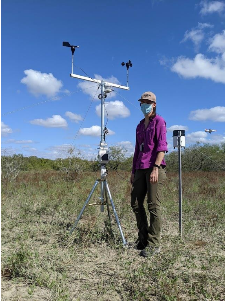
Figure 2. Riparian weather station deployed by Texas A&M University on the northwest end of the airfield at Naval Air Station Kingsville, Texas.
