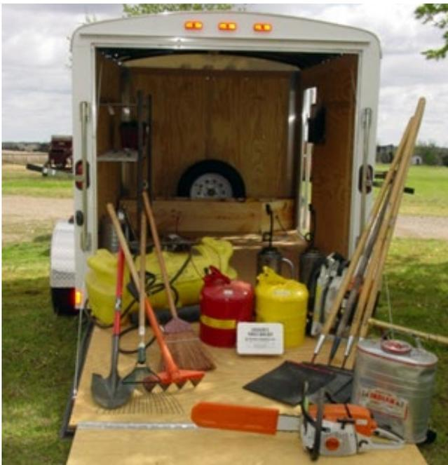
Figure 16. Burn trailer. Photo: Cross Timbers OKPBA
