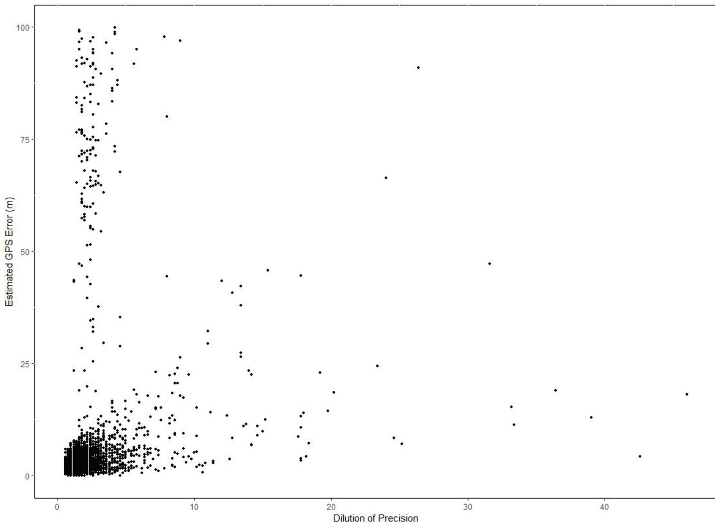
**Figure 3.** Estimated residual error relative to dilution of precision measurements for all PinPoint GPS transmitters evaluated in north-central Texas during 2014 using edited dataset of all residual error locations <100 m.
