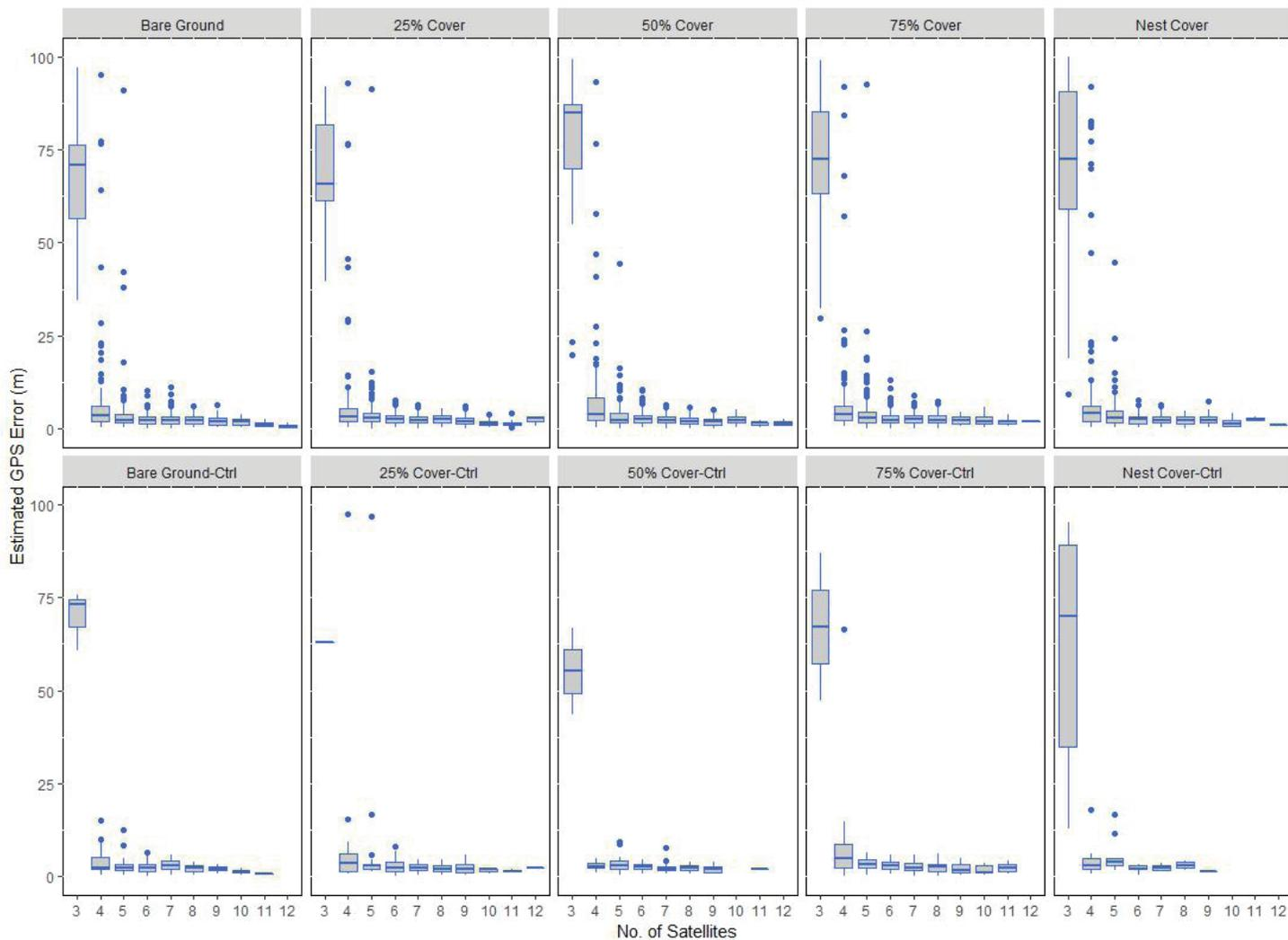
**Figure 4.** Estimated residual error relative to number of satellites acquired for all PinPoint GPS transmitters evaluated in north-central Texas during 2014 using edited dataset of all residual error locations <100 m.
