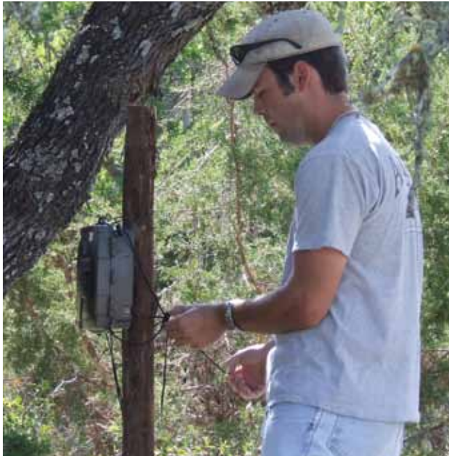
Mount a trail camera to a post or tree approximately 6-10 feet off the ground and placed such that the line of bait is completely visible within the camera's field of view.
